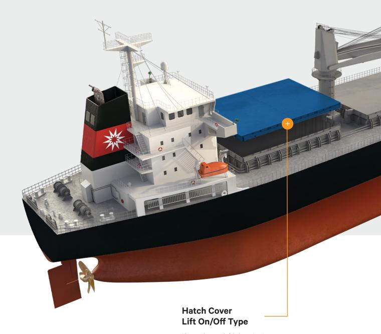
There can be several of deck openings in a ship, serving different purposes but where each opening might pose a threat to the water and fire integrity.
